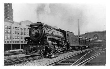
CPR Pacific No. 2715 prepares to haul a Toronto-bound train out of Central Terminal in the mid-1930s. The locomotive was an "international" engine equipped with Automatic Train Control so it could operate over the New York Central. In Toronto, 2715 was serviced at John Street. (Al Paterson photograph)
