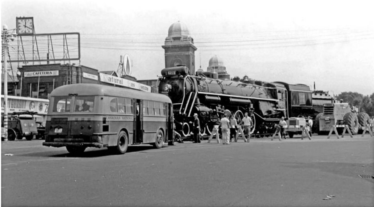
Just after noon on the fourth day of moving to the display location on the CNE grounds. A Canadian National crew bus serves as the lunch room while the foreman (in the straw hat) surveys the task ahead. The Hough loader was used to move 6213 while the air compressor kept sufficient pressure in the loco's reservoirs to provide engine braking if needed. 15 August 1960. John D. Knowles photo
